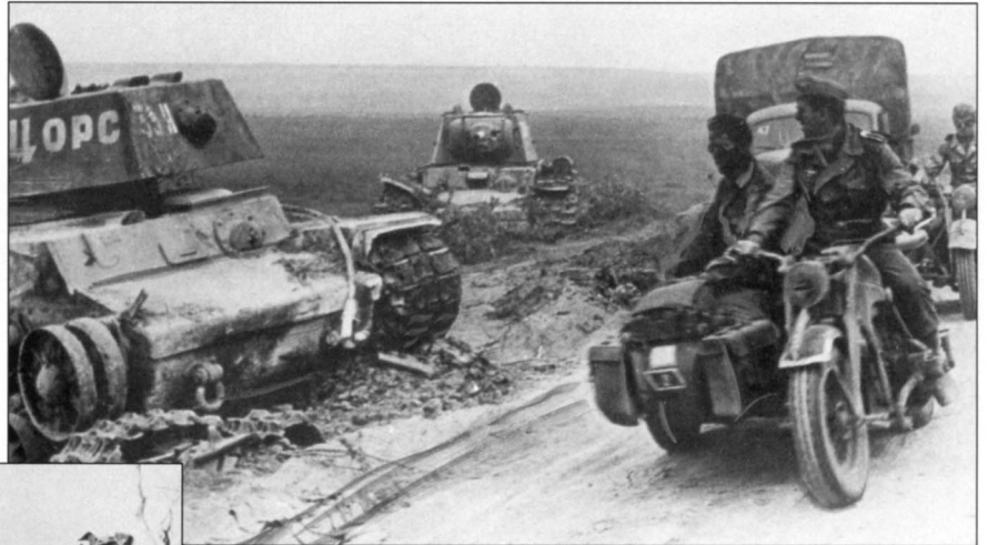
A Pz.Kpfw. III (background) encounters two derelict KV-1 heavy tanks. The strong armor of the Soviet adversary made it almost impossible for German tanks to destroy them. Some reports speak of 40 to 50 direct hits by 37mm and 50mm shells simply bouncing off some KVs. Only heavy anti-aircraft guns were able to deal with them.
