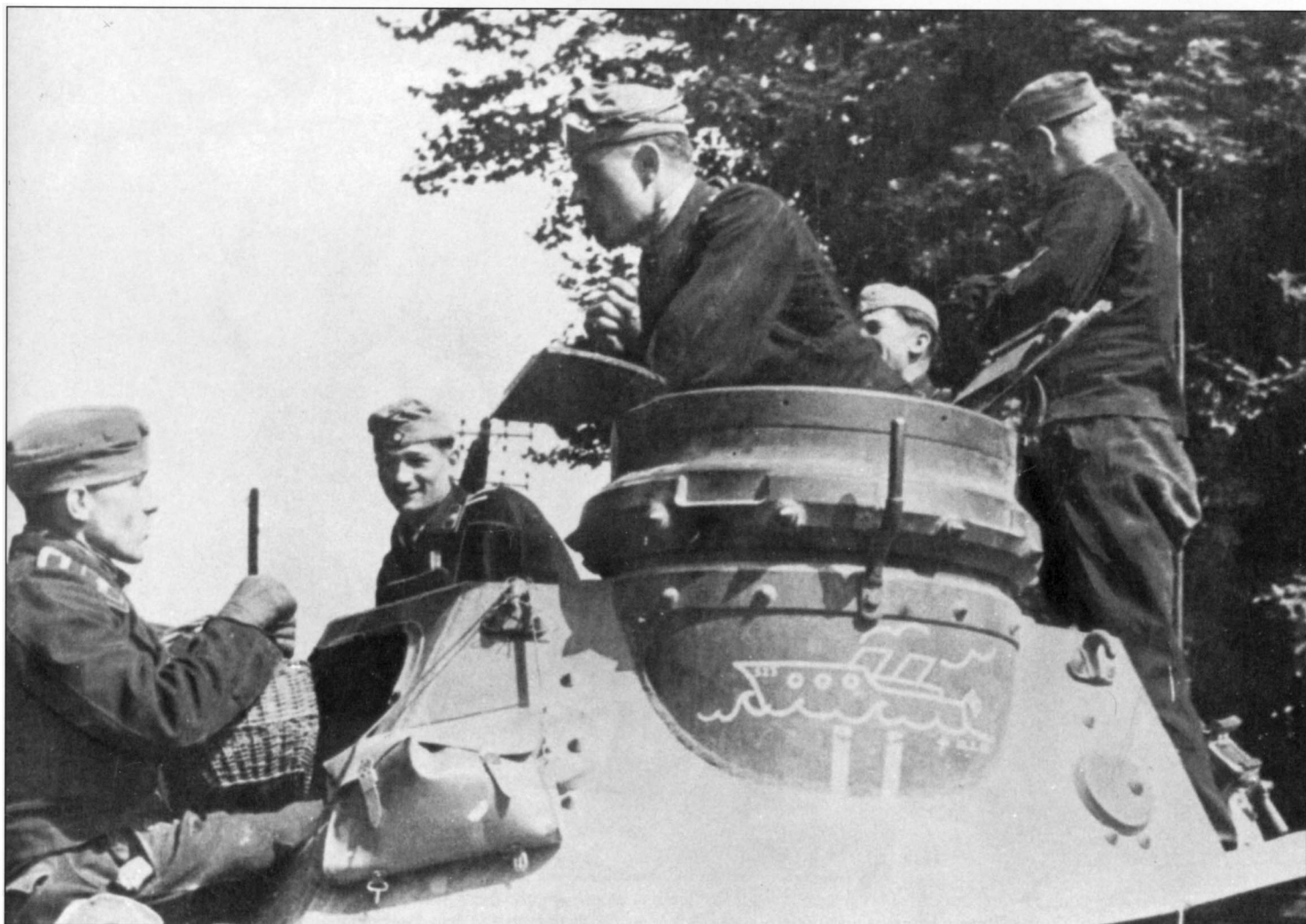
The crew members of a Pz.Kpfw. IV emerge from their tank to take a break. The early commander's cupola is shown in advantage, along with the markings indicating the crew's "kills" — two tanks and a steam ship. Note the mixture of gray and black caps, jackets and trousers worn by the crew.
