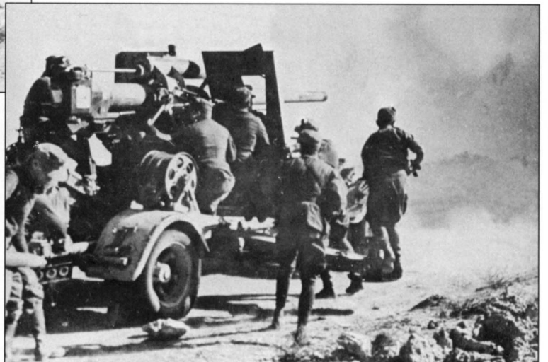
This interesting photo shows an 8.8cm Flak gun in full recoil. Although the practice was forbidden, the gun was sometimes fired from the trailer in an emergency situations. This put excess stress on the carriage and brakes. The gunners wear khaki tropical field caps, headgear that was popular with Afrika Korps vehicle crews.
