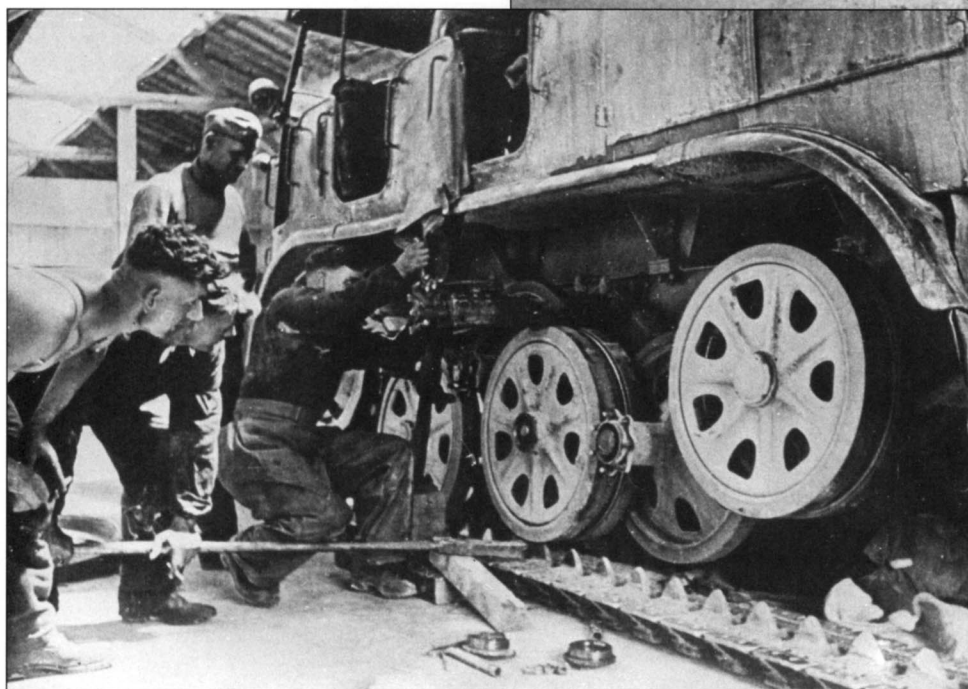
Mechanics perform some maintenance work on an early model 8-ton halftrack. Note that parts of the running gear have been removed. Though the German halftrack prime movers were most successful in their service, they were also complicated pieces of machinery subject to problems, as this photo shows. It is important to remember that none of the armored vehicles of the Panzerwaffe could have operated to its full potential without the assistance of the repair crews.
