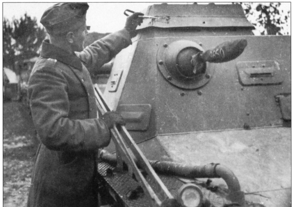
A crew member of this kleiner Panzerbefehlswagen I Ausf. B points to the impact of a machine gun bullet visible on the vehicle's cupola. As humorous as the scene might appear, the photo makes clear that the armor of the light German tanks was very thin; an antitank rifle would surely have ended the service life of this kl.Pz.Bef.Wg. I.
