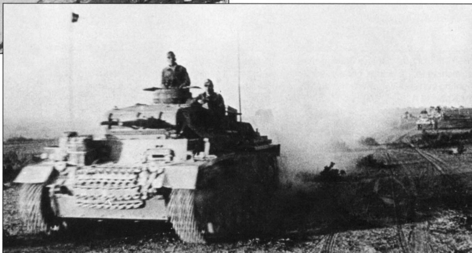
A Panzerbefehlswagen III Ausf. H leads a tank column through the desert. This command tank was fitted with a dummy gun resembling the 5cm KwK L/42. The 2m and the 1.4m rod antennae are both clearly visible; the larger frame antenna on the engine deck can just barely be seen.
