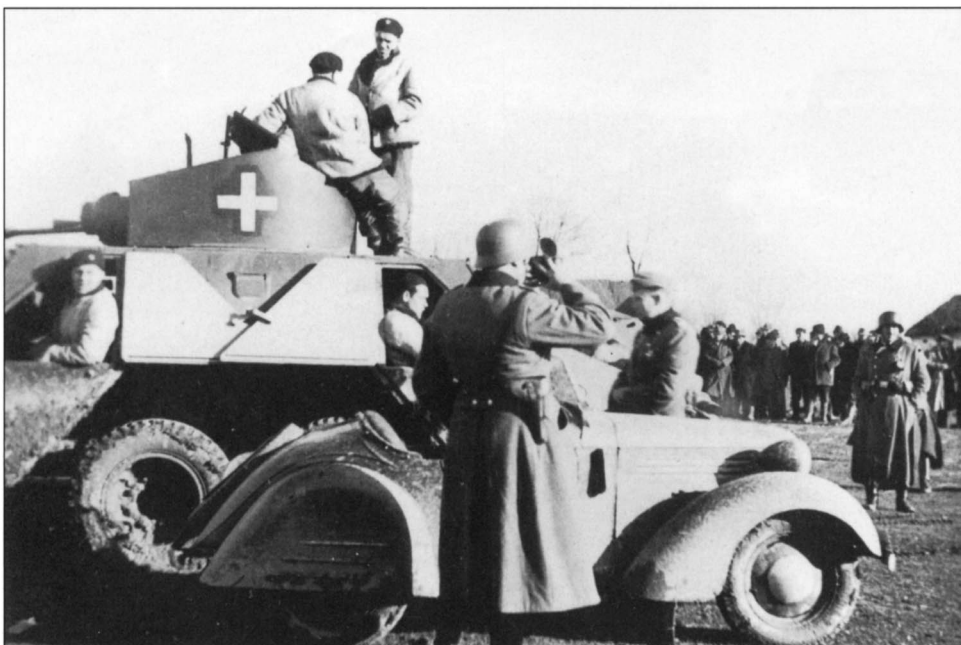
The profile of the ADGZ armored car is shown in this photo. The side hatches are open, illustrating that armor protection was on the lower part of the vehicle. These vehicles were never popular with the German troops. After the first combat in Poland, they were used in an antipartisan role in the Balkans.
