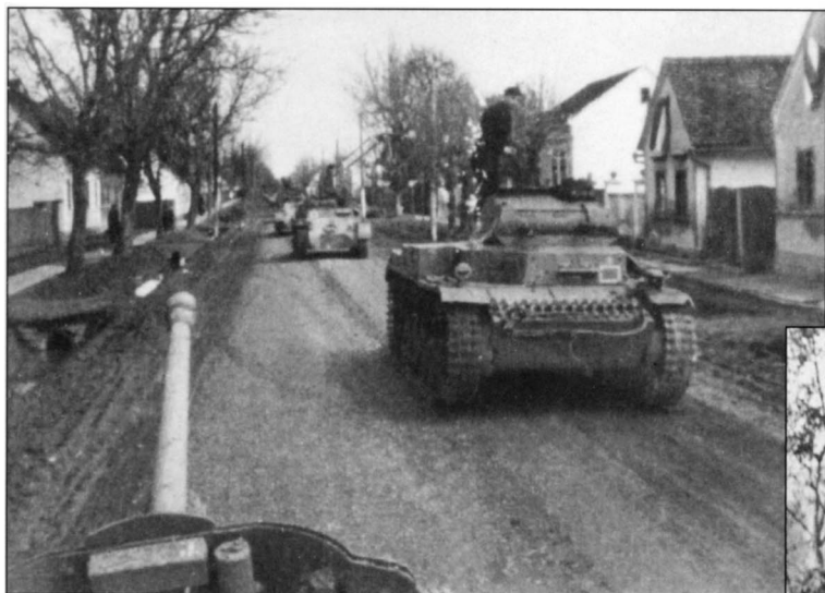
Here a platoon of light tanks passes by an antitank gun unit. The leading tank is a Pz.Kpfw. II Ausf. C; the following is a Pz.Kpfw. I Ausf. B. The 5cm Pak 38 was the most powerful German antitank gun of this period. Basically a very good gun, it became obsolete with appearance of the T-34 medium and the KV heavy tanks.
