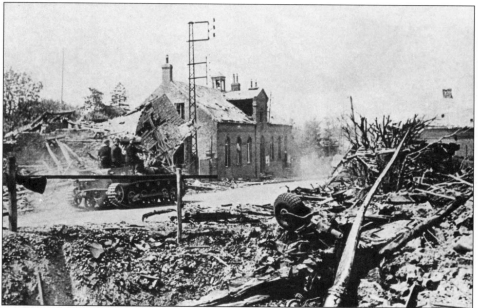
Many Pz.Kpfw. Is were converted to ammunition and supply carriers by removing the turret. While this Munitionsschlepper I (ammunition carrier) passes through a devastated French town, its crew members take a fascinated look at some typical debris of war.
