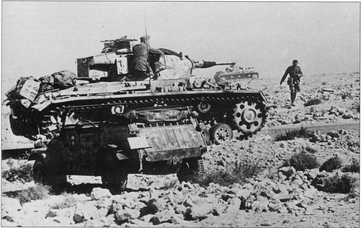
Waiting for action, the crew of this Pz.Kpfw. III Ausf. G looks rather bored. The 5cm KwK L/42 gun has been fitted with a protective covering to prevent dust from intruding into the recoil mechanism. As was a common practice, a lot of extra equipment is stored on the vehicle. This was essential in the desert. The tank has apparently been camouflaged with the application of irregular yellow stripes over the gray base color. The dust would have further improved the camouflage. Note the tactical markings and the splotchy appearance of the Kübelwagen in the foreground.
