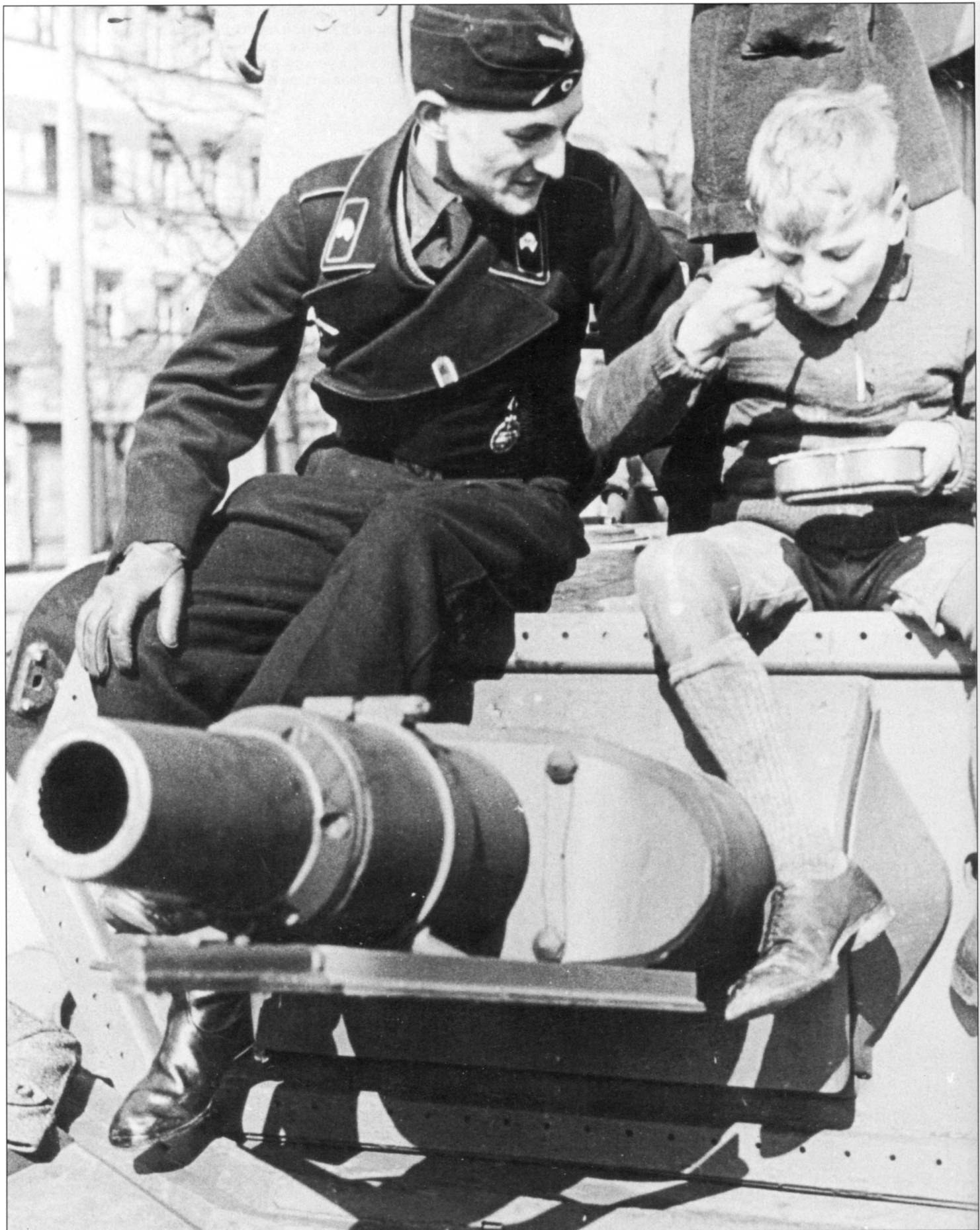
This interesting shot shows a tank trooper sharing rations with a young boy atop a Tauchpanzer IV wading tank, which is identifiable by the perforated frame mounted on the turret's front plate. The gun and deflector are clearly visible in this photo. With Operation "Sea Lion" abandoned, the bulk of the Tauchpanzer s went to 18. Panzer-Division, which crossed the River Bug underwater on 22nd June 1941. For uniform enthusiasts, this close-up shows an early pattern jacket with piped collar and the black Feldmütze sidecap, which was being issued by the time of Operation "Barbarossa".
