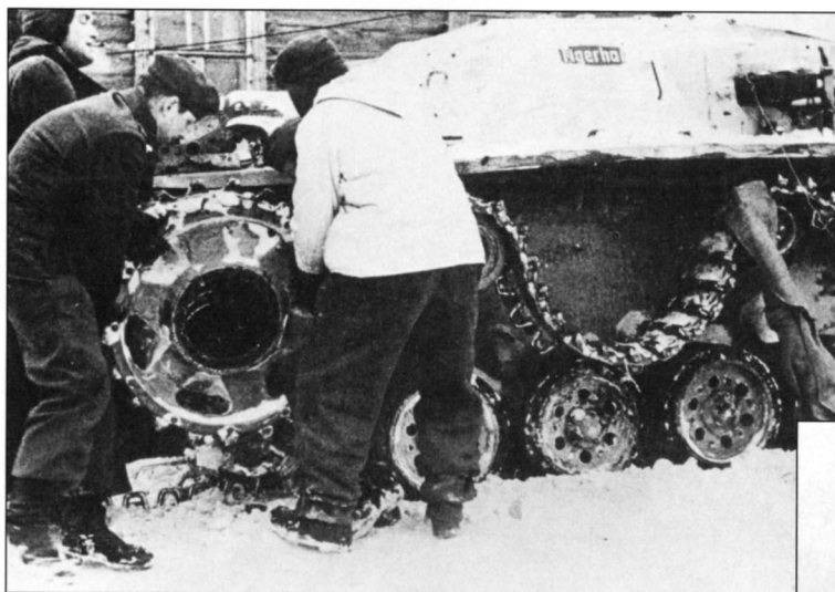
Here the crew of a whitewashed StuG III Ausf. E changes the track, possibly because of damage inflicted by a mine. Note that the vehicle was given the name "Leopard", a practice that was common among assault gun units. The vehicle is loaded with a lot of personal gear and spare parts.
