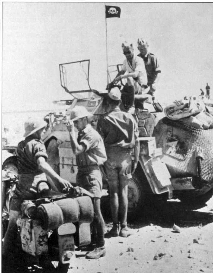
The commander of 15. Panzer-Division reconnaissance company gives new orders. The 2m rod antenna on his Sd. Kfz. 222 has been adorned with a pennant showing a Totenkopf , the Death's Head symbol of German tank units. The amount of extra equipment that has been packed onto the armored reconnaissance vehicle is noteworthy. The Zündapp KS 750 motorcycle seen at left was used as a liaison vehicle.
