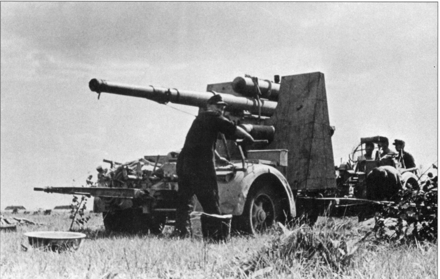
A crew member lowers down the rear support of an 8.8cm Flak 18. The AA guns used in ground combat were often not camouflaged since they could rely on their long-range antitank capability for protection. Further, sometimes the course of a battle did not allow this luxury.
