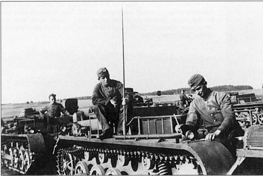
Another Fahrschulwagen driver training vehicle belonging to a different unit. This one, which is finished in plain dark gray, is fitted with a radio for training purposes. At the beginning of WWII the Germans had a highly trained tank force thanks to the availability of these light tanks.
