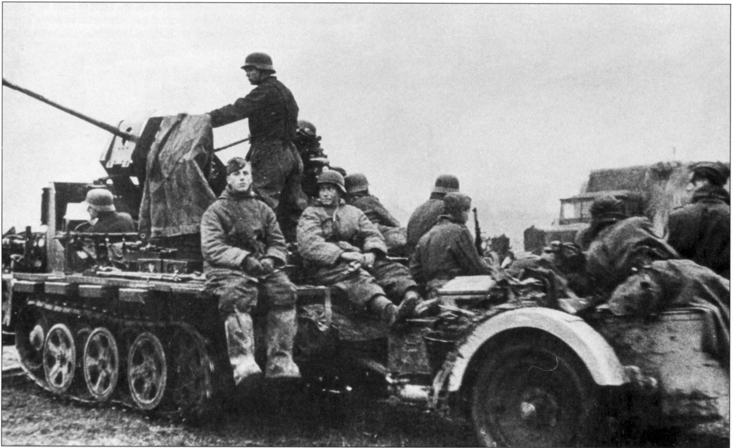
This Sd.Kfz. 10/4 shows a partly armored driver's cabin. These versatile vehicles were often used near the MLR for direct fire support for infantry units, a task they were not intended for. The inadequate armor protection resulted in heavy losses. Note the heavy winter clothing worn by the soldiers.
