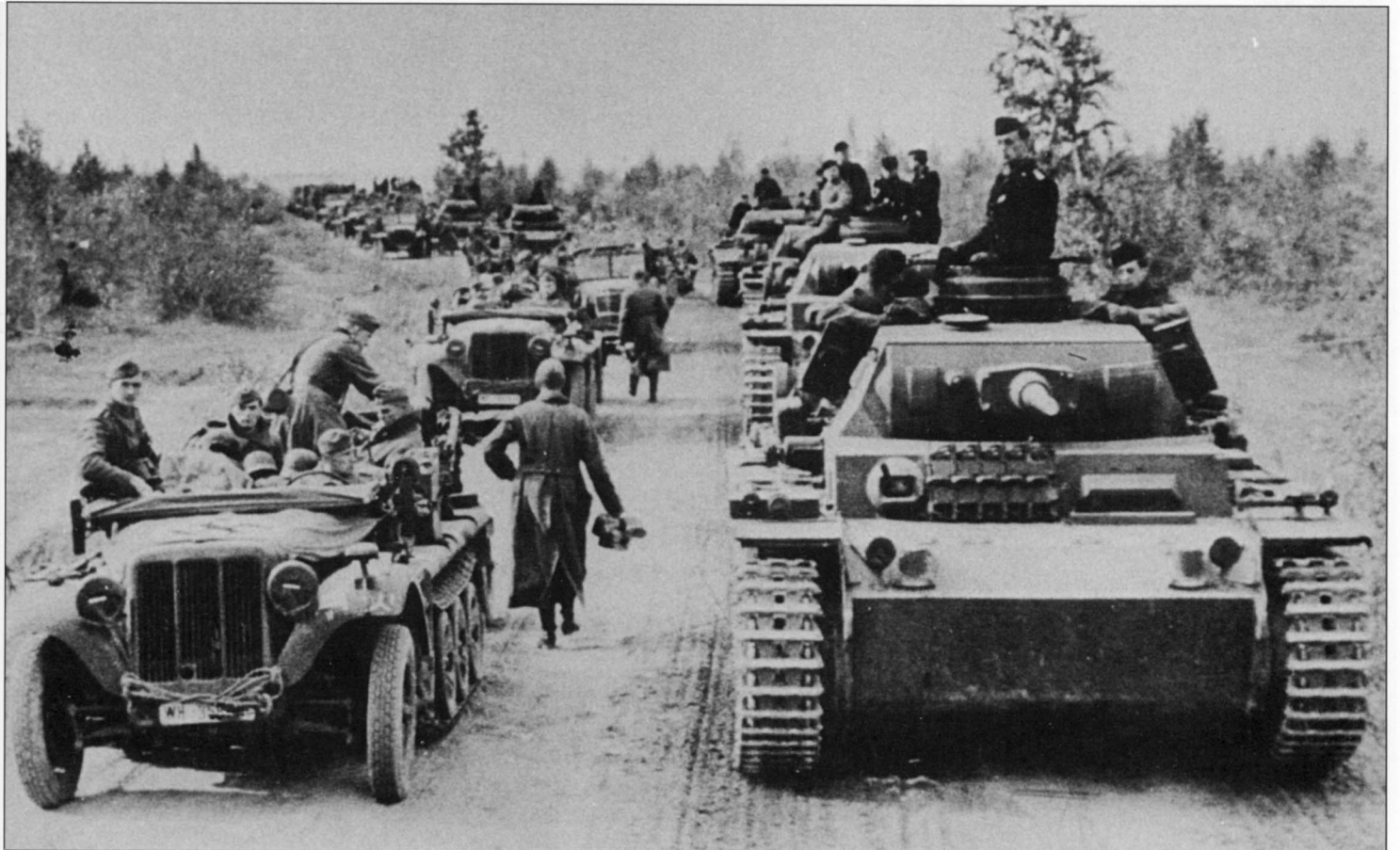
A mixed column of tanks and halftracks advances up a road. The Pz.Kpfw. III in the foreground is from an early Ausf. J production lot, as is evident by the ball-mounted MG 34 in the front of the hull. The Ausf. J featured many improvements, such as thicker armor on the superstructure, that were made based on combat experience.
