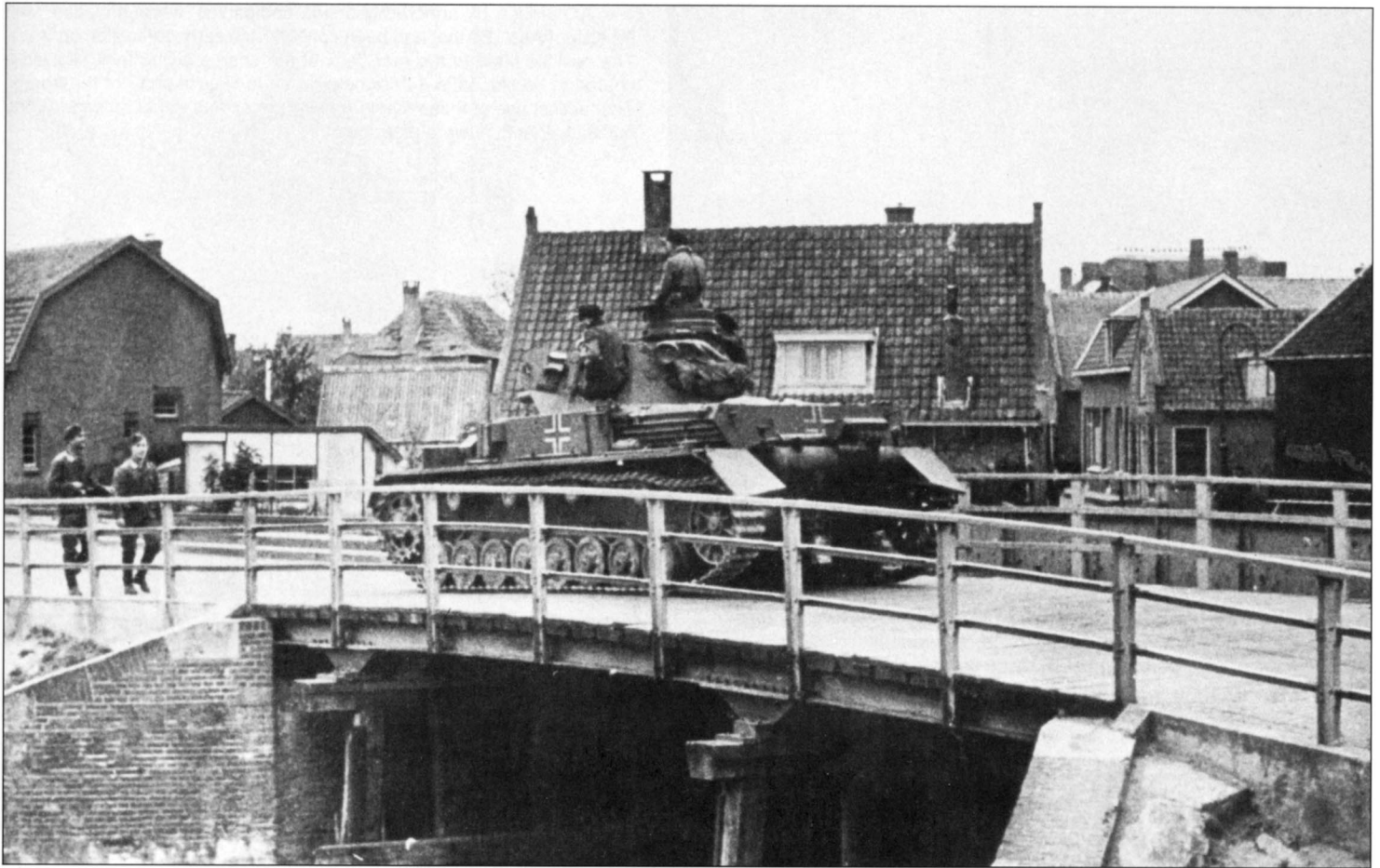
This Pz.Kpfw. IV Ausf. D crosses a bridge in the Low Countries in 1940. The tank wears the narrow white German crosses that were commonly seen during the Western campaign. It is also equipped with five smoke candle dischargers, which was typical for German tanks and StuGs in that year.
