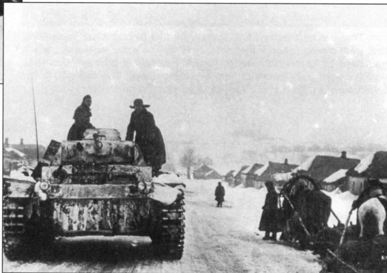
This whitewashed Pz.Kpfw. III Ausf. J encounters Russian peasants escaping from the front line. Although it was planned that the Ausf. J would be equipped with the 5cm L/60 gun, production delays prevented this from happening. So, the first production batches left the factories with the less powerful 5cm L/42 gun. This tank sports a rather scruffy winter camouflage.
