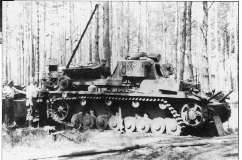
A damaged Pz.Kpfw. IV Ausf. E is being repaired in a forest workshop. Though its drive sprocket is broken, the vehicle was kept in running condition by repositioning the track around the frontal return roller and running wheel. A large crane, possibly mounted on a tank, is removing the engine.
