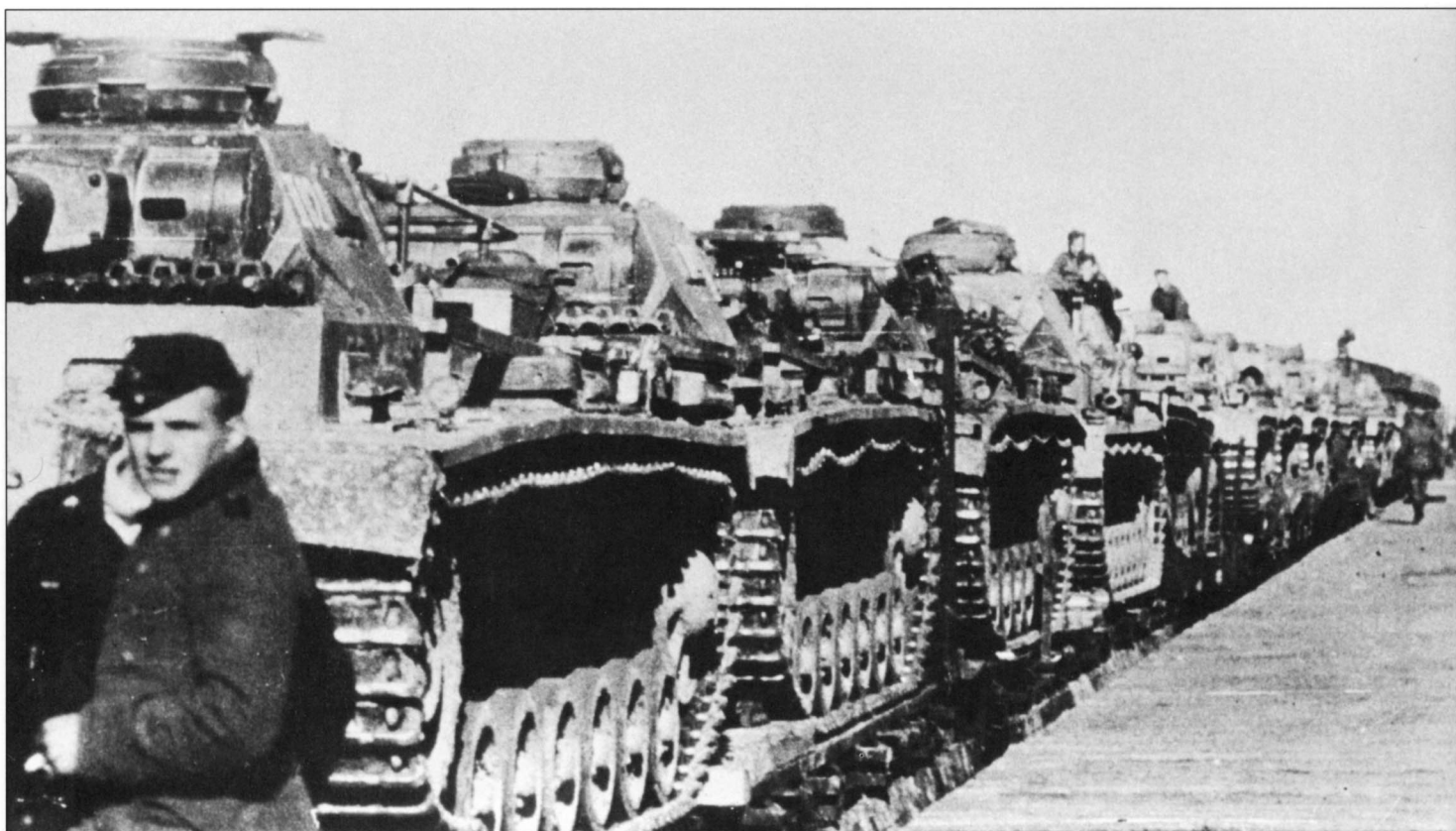
A tank unit, possibly part of 10. Panzer-Division belonging to Heeresgruppe Mitte, waits for railway shipment to the front. The first three vehicles are Panzerbefehlswagen III Ausf. H command vehicles, possibly belonging to the battalion staff section. These command tanks have been disguised with a fake 5cm KwK L/42 gun.
