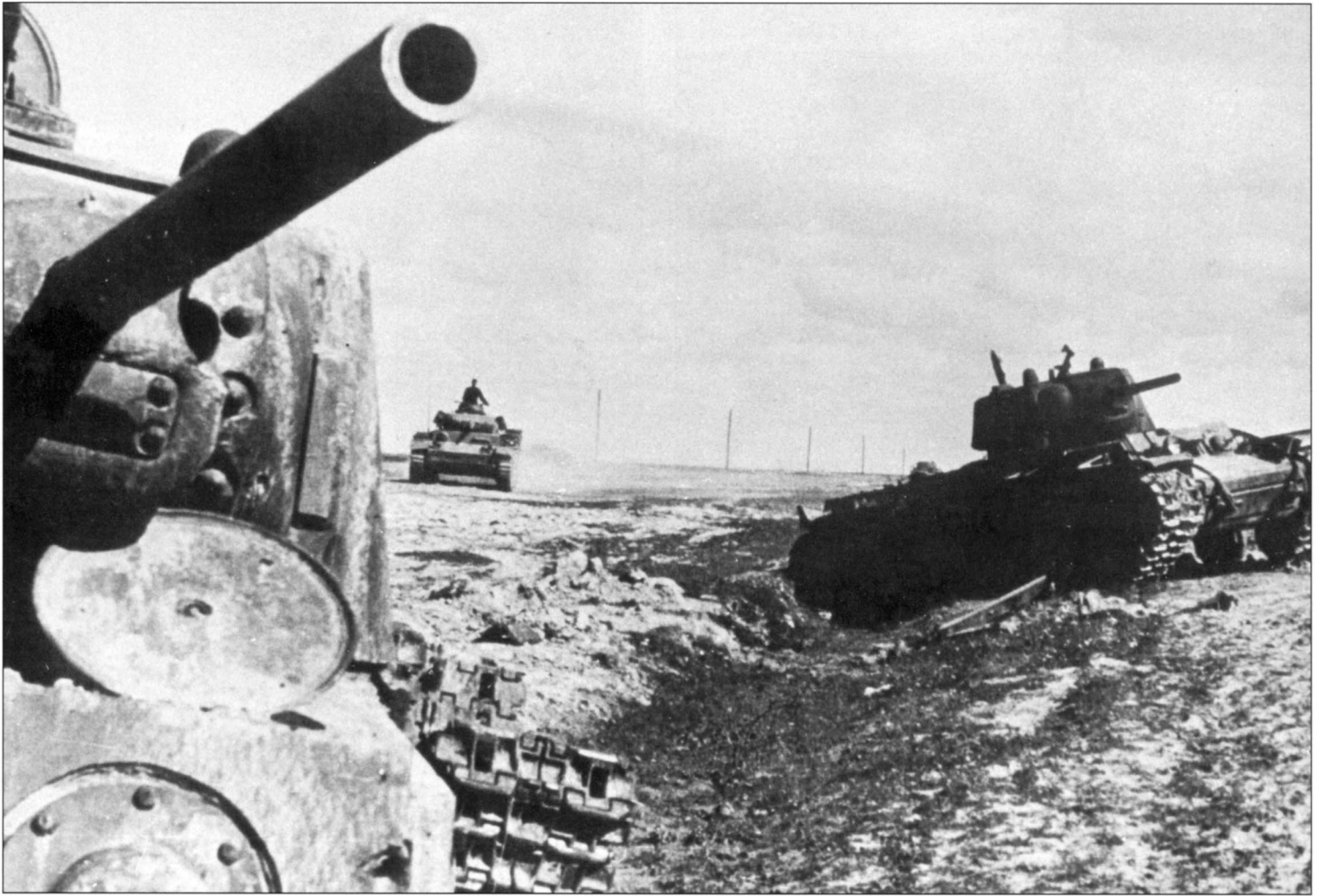
A Pz.Kpfw. III (background) encounters two derelict KV-1 heavy tanks. The strong armor of the Soviet adversary made it almost impossible for German tanks to destroy them. Some reports speak of 40 to 50 direct hits by 37mm and 50mm shells simply bouncing off some KVs. Only heavy anti-aircraft guns were able to deal with them.
