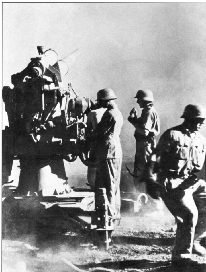
This 8.8cm Flak gun is being used in a more traditional artillery role as it provides support fire during an advance. One gunner can be seen standing at the gun looking at his Folgezeiger data transmitting system, while the commander supervises the action. It is noteworthy that the gun has no shield, leaving the crew without protection.
