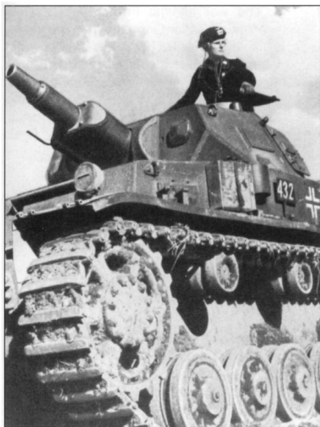
This well-known propaganda photo shows a Pz.Kpfw. IV Ausf. B or C of Pz.Rgt. 7, 10. Panzer-Division, as is indicated by the silhouette of the charging Bison stenciled on the lower left of the turret. The short-barreled 7.5cm gun is shown to advantage here. Also of interest is the antenna deflector attached to the gun.
