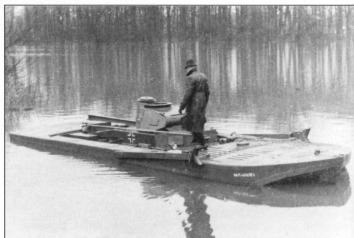
Shortly after the invasion of France, the Germans prepared for the planned invasion of Great Britain. This photo shows a prototype of the Schwimmpanzer II, a Pz.Kpfw. II Ausf. C that is carried through the water by a large pontoon. Equipment like this was later used along with deep-wading tanks during Operation "Barbarossa".
