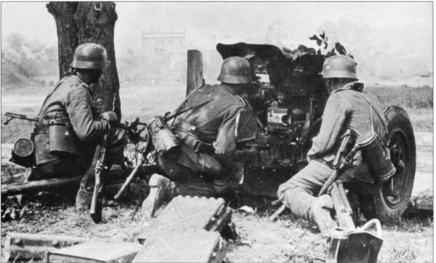
The 3.7cm Pak 35/36 was a good gun — by 1934 standards. However, by the time of the campaign in the West, it had already shown that its armor penetration was too weak. Hopelessly outclassed and ineffective in the East, the 3.7cm gun was nicknamed Heeresanklopfergerät — door knocker— by the German troops.
