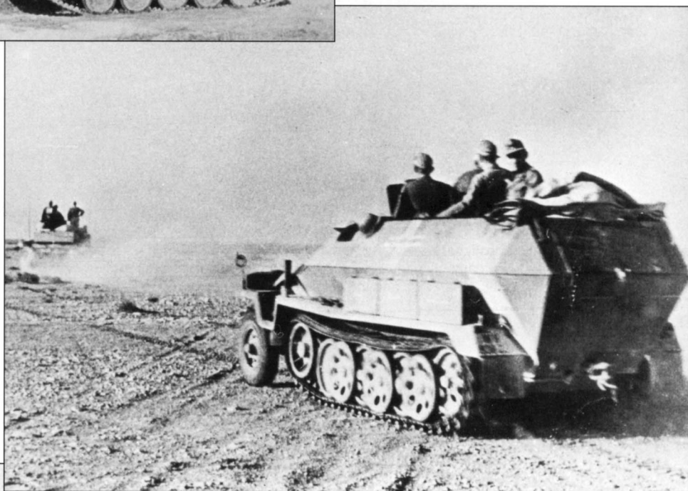
A Sd.Kfz. 251/1 Ausf. C, with a welded body, follows a Pz.Kpfw. III through the open desert. The vehicle is finished in sand yellow and displays a prominent national insignia. The armored halftracks were very versatile, but the German war industry was never able to produce a satisfactory number of these vehicles.
