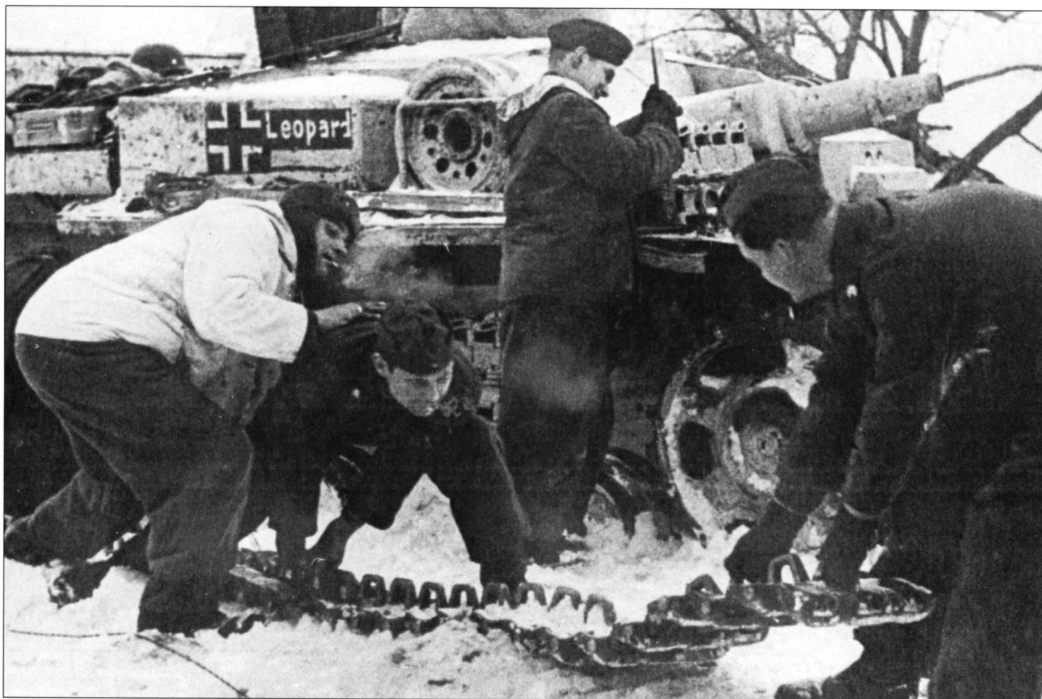
Here the crew of a whitewashed StuG III Ausf. E changes the track, possibly because of damage inflicted by a mine. Note that the vehicle was given the name "Leopard", a practice that was common among assault gun units. The vehicle is loaded with a lot of personal gear and spare parts.
