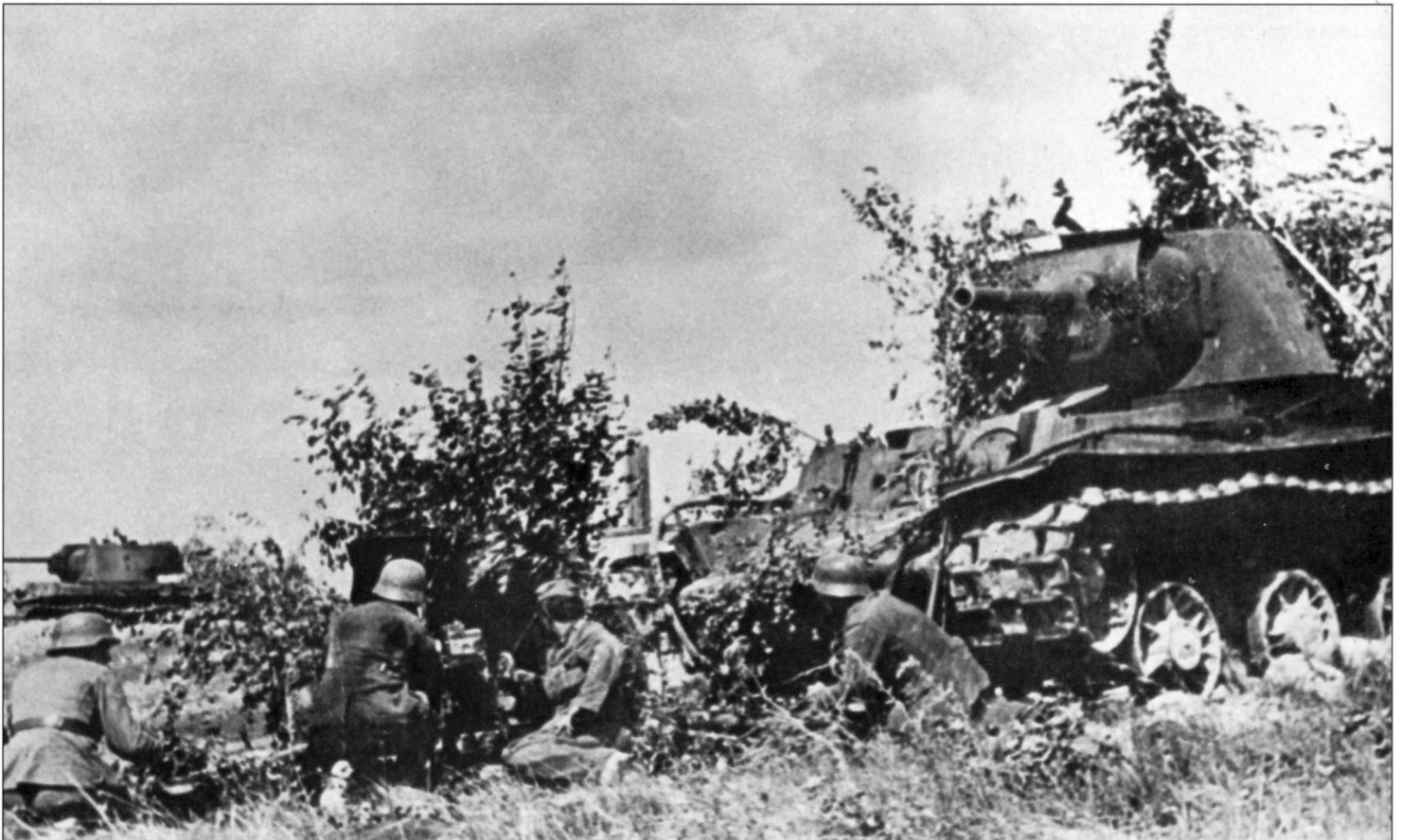
A thoroughly camouflaged 3.7cm Pak gun in attack position in the shadow of a KV heavy tank. The technical manual for the antitank gun said that the Soviet heavy tanks could not be destroyed. It was supposed to be possible to put the tank out of commission with a few well-aimed shots into the optics or the drive sprockets.
