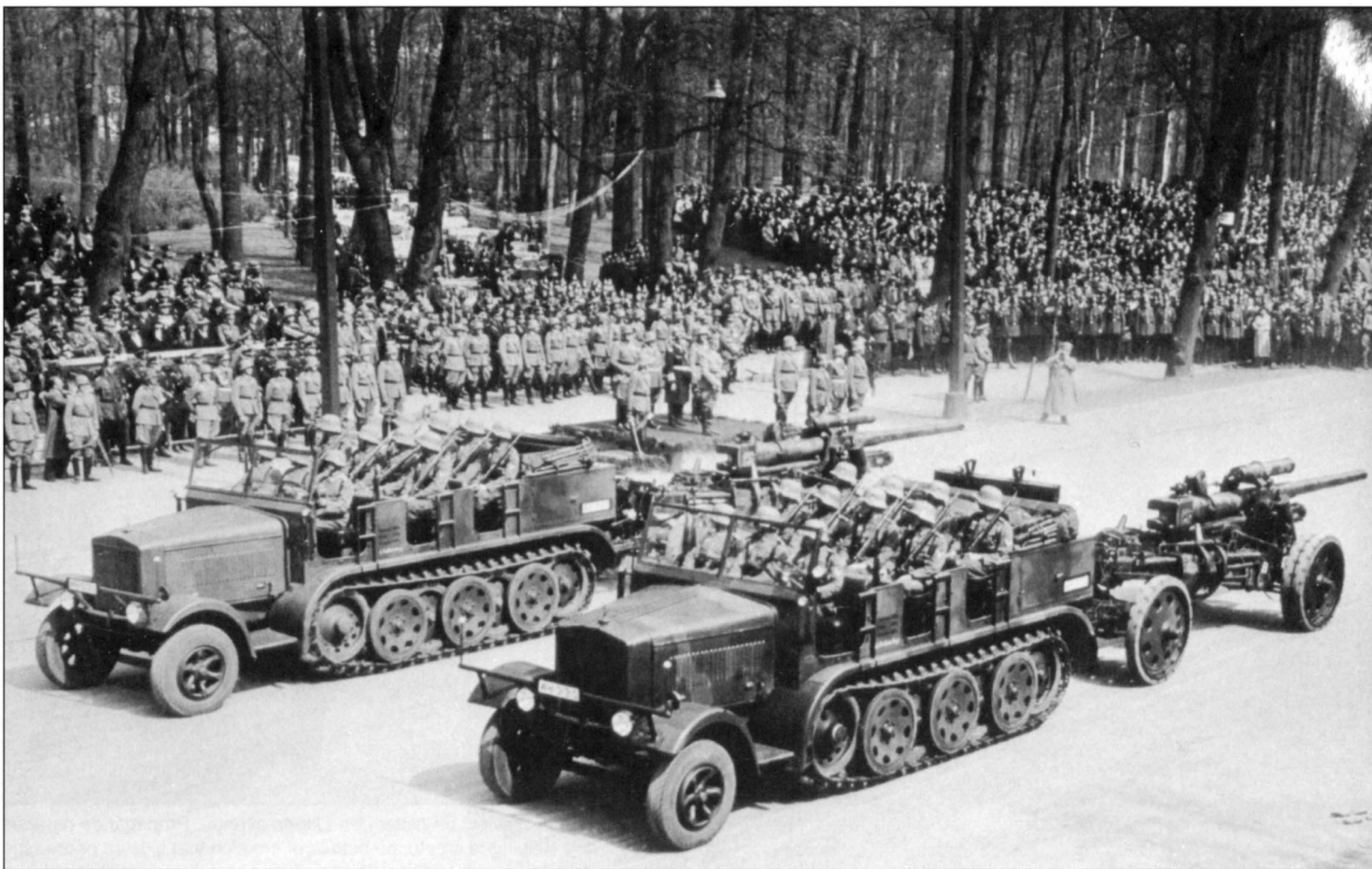
Two heavy half-tracked prime mover tractors (12-ton Zugmaschine , DBs 7, Sd.Kfz. 8) haul troops and tow guns (s.10cm Kanone 18) during a parade. These halftracks offered outstanding cross-country maneuverability combined with high road travel speed and were an integral part of the Panzer division.
